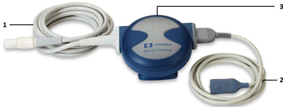
Figure 3: BISx4™ - 1- Monitor Interface Cable connects to Monitor; 2- Patient Interface Cable connects to BIS™ sensor; 3- BISx4™ (BIS™ LoC 4 Channel)
