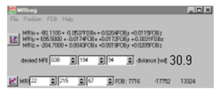
Left: Example of Steps 8 & 9. The 'desired MRI boxes' are displayed. Additionally, the current distance of the magnetic sensor from the coordinates entered in the 'desired MRI boxes' is displayed, which in this example, is 30.9 mm.
